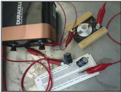
In series: (2) 2200 \mu F capacitors, 6 V battery , 1.3 V bulb.
